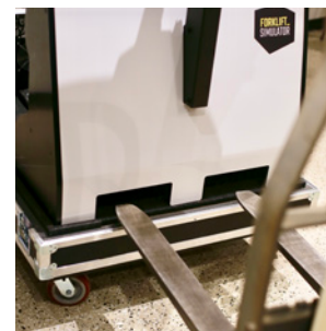
4. Lift the Forklift Simulator and roll the bottom case underneath the Forklift and slowly set it down.
