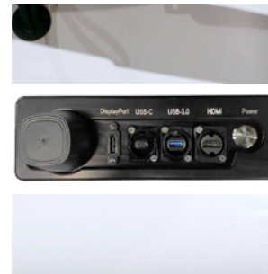
1. Shut down the unit by pushing the power button once.
