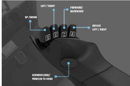
Calibration functions using the control handle.
