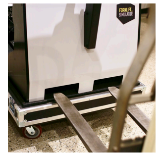
5. With a forklift, evenly align the forks to the entry points of the Forklift-Simulator. Lift the Forklift Simulator several inches above the flight case so that you can roll the flight case out of the way. Once the flight case is removed, slowly set the Forklift-Simulator to the ground. From this point on you can easily move the unit around using a hand pallet.
