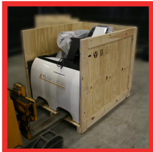
4. Using a forklift (or similar device) lift the unit by its fork pockets and remove the crate by sliding from underneath the unit.
