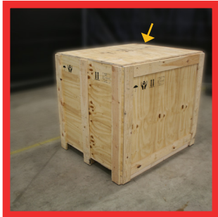
1. Remove the screws that hold the top lid and remove it.
